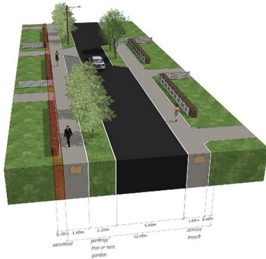
Figure 4 - Minor Residential Road
